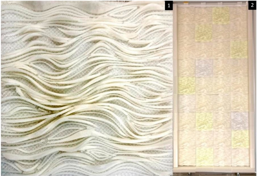
Figure 3. The urban screen system is designed for hosting the bioluminescent bacterial strain A. fischeri for integration in the built environment and in architectural and urban applications. 1. One 3D-printed bioreceptive tile of the bioluminescent urban screen, showing the varied topology between peaks and wells and interstitial spaces, as well as the micro-textured square grid for better anchorage of the hosted bacterial strain. 2. A fully assembled urban screen panel measuring 170 × 90 × 4 cm, incorporating the 3D-printed tiles with varied PLA filaments between translucent, transparent, and fluorescent, which will be tested for their effect on the bioluminescent activity of the hosted in A. fischeri and exhibited in a future study.
