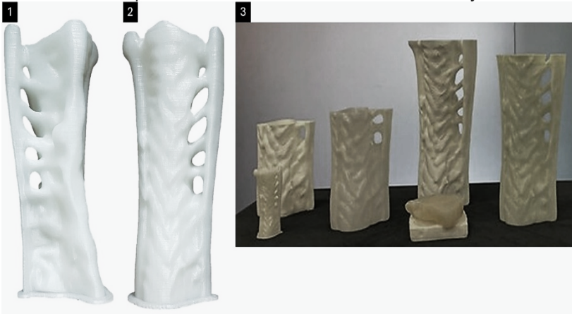
Figure 16. The bone-shaped biocontainer for bioluminescent liquid culture. 1. and 2. are two views for the 1:10 scaled model of the bone shaped biocontainer. 3. is the 3D printed models of the 1:2 scaled biocontainers in different printing stages and with varied PLA filaments including translucent, transparent and luminous filaments. The photo is taken from the Heart of Architecture Exhibition, held at Universitat Internacional de Catalunya, Barcelona, February 2025. By the authors.
