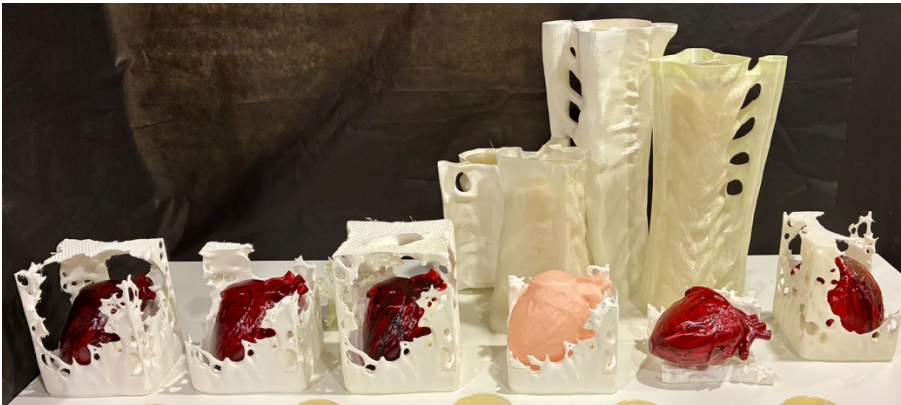
Figure 14. The Urban Hearts Biocontainers and MFC chambers 3D printing and colouring: varied scales of the 3D printed heart biocontainers. 1. Is the urban scale 3D printed heart biocontainer of (40 x 40 x 50 cm) 3D printed in translucent red PLA using the Felix XL pro dual head printer. 2., 3., 4. exhibits the architectural element scale heart biocontainer of (20 x 20 x 20 cm) 3D printed in translucent red PLA using Felix Pro Dual Head printer and finished with varnish (translucent carmen red and translucent) to conceal any pours and give the realistic effect of heart capillaries and blood mimicking the human heart. 5. and 6. are two views of the dried urban heart biocontainer on a 3D printed stand which is part of the Heart Shelter Brick. Below the Urban Hearts and Bone Biocontainers in the BioLumCity exhibition. By the authors.
