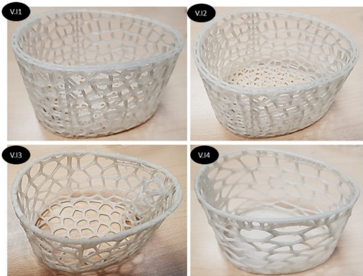
Figure 9. Four different iterations of the Voronoi design family of the biocups. V.I1 exhibit the first design iteration using tight straight double walled Voronoi structure of 500 points population as base for the 3D Voronoi structure (exhibiting the top view plan, perspective and left side view), enhanced to V.I2 with less density, wider double walled Voronoi structure of 300 points population base of the Voronoi structure. V.I3 exhibits the shift to curvy (chamfered) single-walled hollow pipes Voronoi structure with 150 points population of the Voronoi structure evenly distributed, while V.I4 is adding attractors of the Voronoi structure towards the borders of the biocup as an emphasize on the horizontal ends of each biocup. However, this iteration would result in uneven exposure of the immitted bioluminescent light, blocking light at the bottom and top of each biocup and resulting in lesser light amount. Thus, iteration V.I3 was the one chosen for further customization and application in the biolamps.
