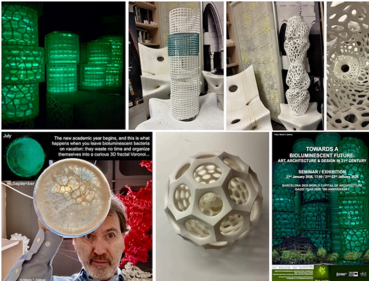
Figure 12. From left to right, the final family of Voronoi biolamps, the grid biolamp, the biocolumn, and below bacteria self-organized in Voronoi after two months growing, the radiolarian biolamp and the exhibition poster: all digitally designed and 3D printed for bioluminescence domestic and urban use. By the authors.
