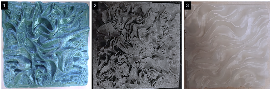
Figure 7. design variations for the bioreceptive panels, varying the design based on customizing fields-based patterns with differential growth patterns, also varying the colour, transparency and reflectivity of the used PLA filament in the 3D printing process of each of these design variations. By the authors.
