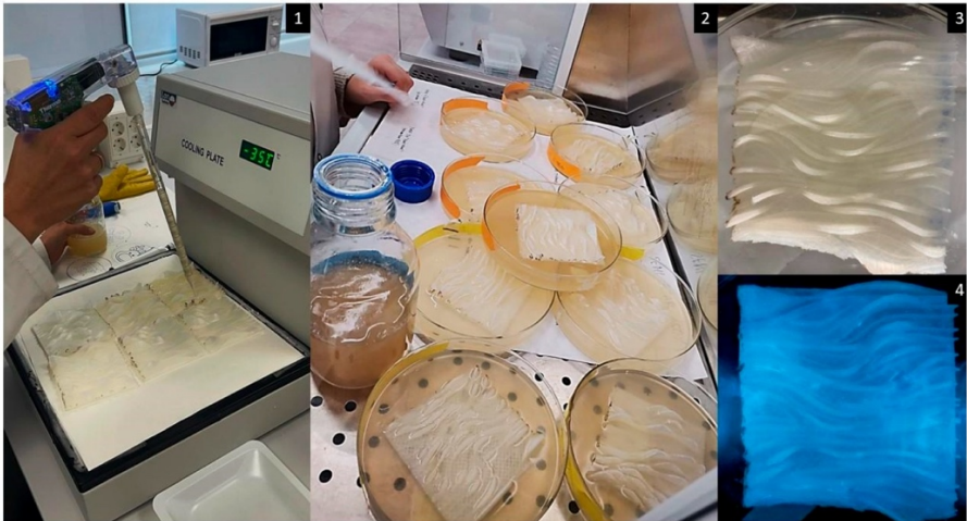
Figure 6. The bioluminescent urban screen culturing and bioluminescence activity: 1. Cold-plate freezing of the 3D-printed tile, divided into four parts, for sterilization and preparation for adding the slurry culture of the bioluminescent bioink. The seeding process was followed by covering it with the media in 5 layers. 2. The seeded urban panels' parts cultured in petri dishes. 3. The P1 part of the urban screen panel seeded with the bioluminescent bacterial culture + media in agar. 4. The same part under a conventional digital camera with an exposure time of 10 sec. in a dark room (as a naked human eye see it), exhibiting the visible bioluminescence activity, which lasted for 10 days without refilling. By the authors.
